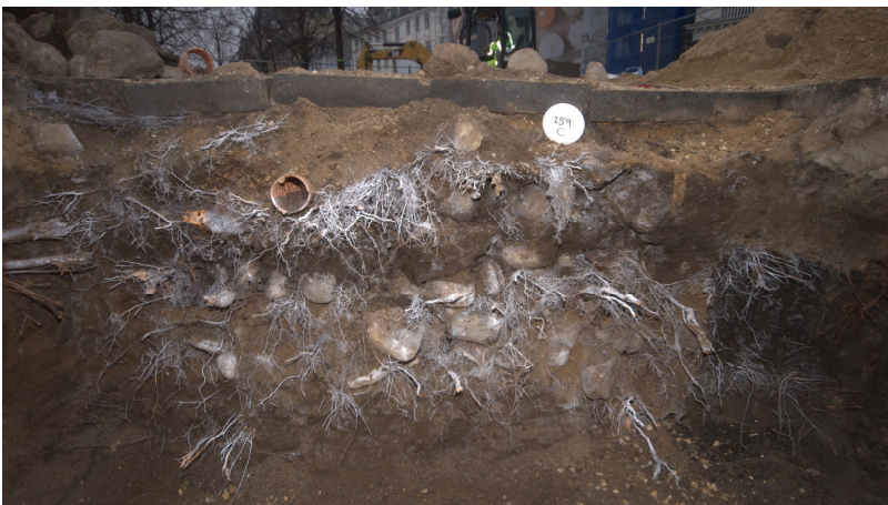
Figure 1: Example of a structural soil profile. For increased visibility, roots have been spray painted.
