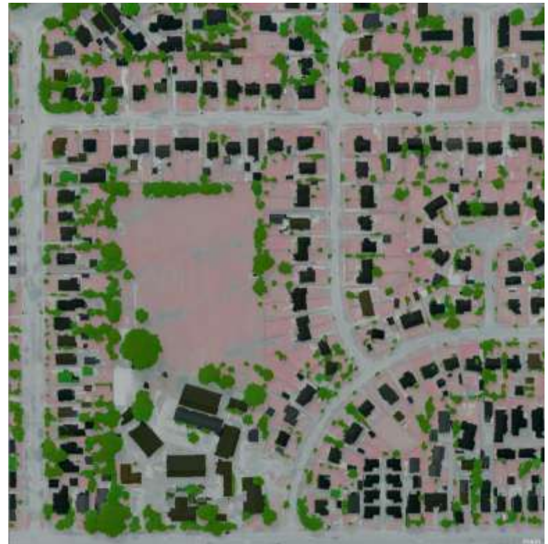
Caption - Example of canopy cover classification using Trimble eCognition software
