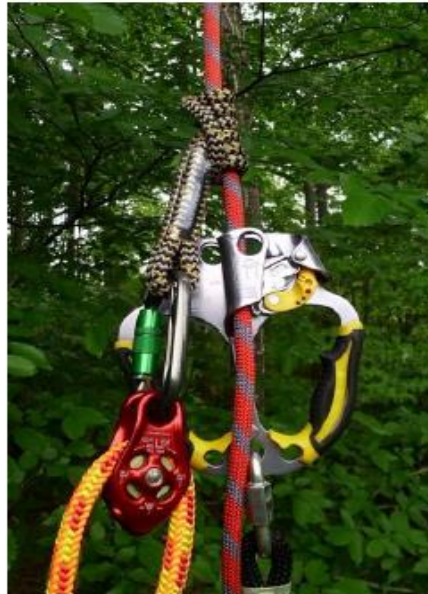
Back-up system attached above highest ascender to access line with friction hitch
