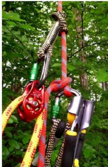
Access line locked off to allow climber to work from climbing line during ascent.
