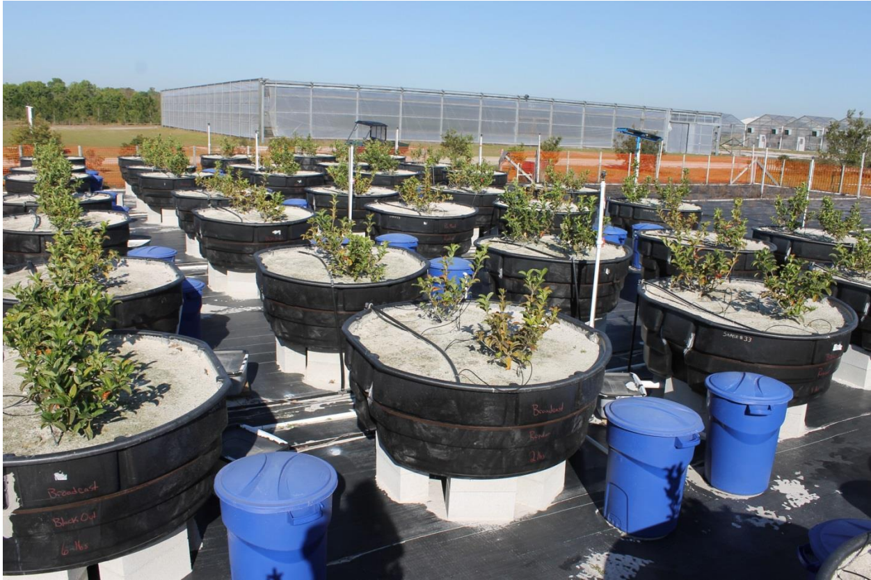
Fig.1. Sweet viburnum ( Viburnum odoratissimum ) planted in elevated lysimeters. Leachate from each lysimeter was pumped into an adjacent collection tank for sampling. In the absence of rain, supplemental irrigation was supplied by a spray stake (01SSBK-B, Netafim USA, Fresno, CA) irrigation system.
