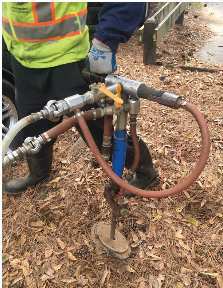
Figure 6. Pneumatic and hydraulic fracturing combined with biochar injection open and stabilize soil pores.
